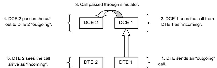
The process is reversed for a call in the opposite direction (i.e. DTE 2 to DTE 1).
