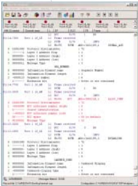
The V5 analyser provides full analysis of all the active C-channels in both the direction of the LE and the AN. V5 and ISDN messages are displayed in the analyser window with decoding for Layer 1, Layer 2, Layer 3 and detected DTMF digits. Messages can be displayed either as full, identified or hexadecimal format and the use of protocol filters allows you to filter out unwanted messages.
